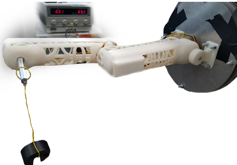
Figure 45: Image detailing how load testing was carried out
