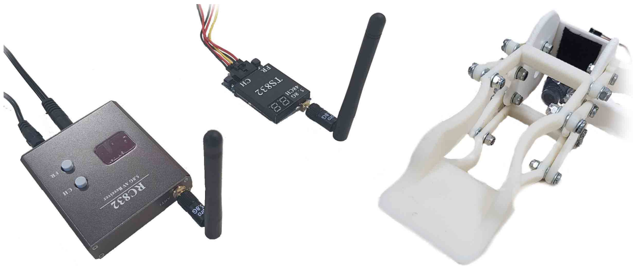
Figure 38: FPV setup components: including the receiver, transmitter and camera inside claw of gripper
